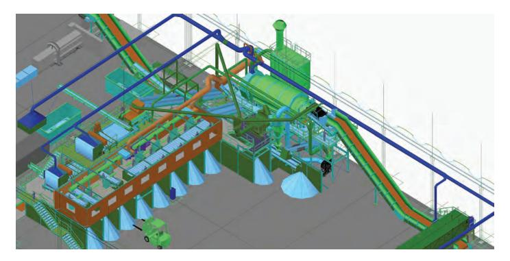
Plants of this type are also used for the selection and increase in value of the residual dry part of the municipal waste deriving from the separated collection; in this way, besides obtaining a reduction of the 30% of the quantity of waste to destine to the dump, considering the consequent prolongation of the residual life of the same, it is possible to obtain an increase in value of the different typologies of municipal waste.
